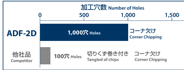
100穴加工後の比較 Comparison after processing 100 holes
